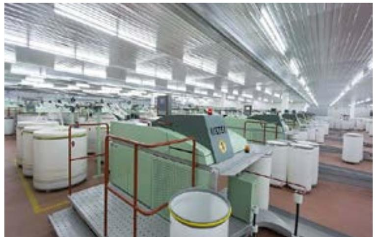
Figure: A high-performing draw frame is the cornerstone of any spinning mill. Courtesy: Rieter
