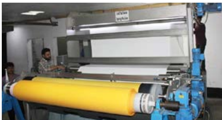
Figure: Robintex's Cold pad batch dyeing system achieves 13% carbon savings and over 50% water savings in fabric manufacturing compared with the conventional exhaust dyeing.
